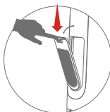
① Clean the filter once a week, put it back after drying.
